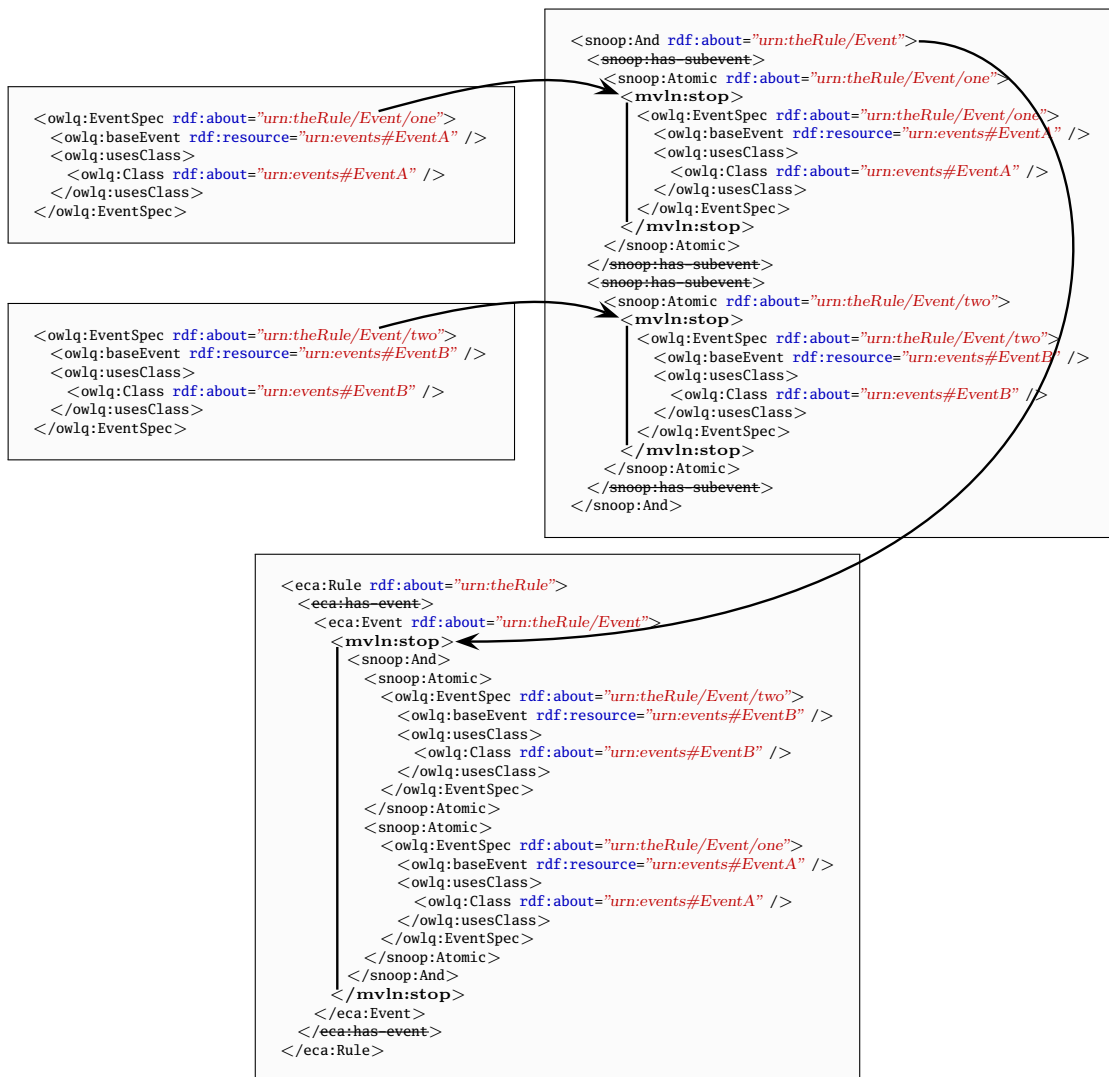
Figure 4.6: The Converted Parts of the Event Component, Stripped and Reattached to the Respective Outer Element Nodes, Wrapped Inside a <snoop/> Element
